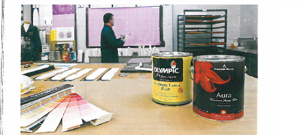
DNE-COAT HIRING Olympic Premium and Benjamin Moore Aura have lower VOC levels than other tested paints and did a good job in this hiding test.
